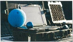
Pipe Diver Ultra: Ultrasonic free-floating sensor assembly scans pipe while being pushed with water flow
